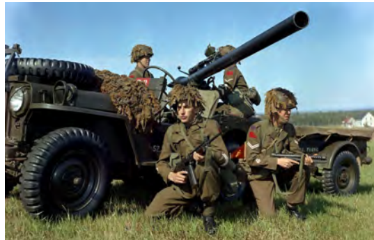
105-mm M40 Recoilless Rifle mounted on a jeep, back in the day. The soldier kneeling on the left is armed with a 7.62-mm FNC2 and the Corporal on the right is armed with a 9-mm Sterling SMG. (Library & Archives Canada
