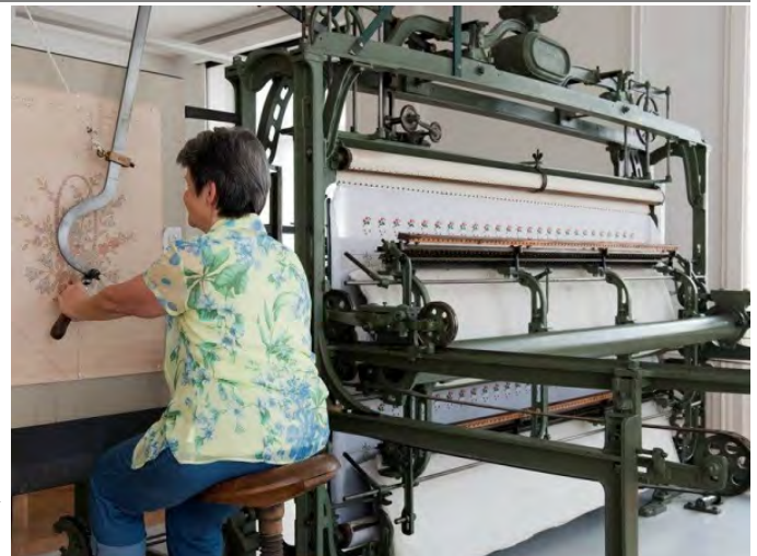
Woman operating the pantograph of a hand embroidery machine, Textilmuseum St Gallen. Switzerland
